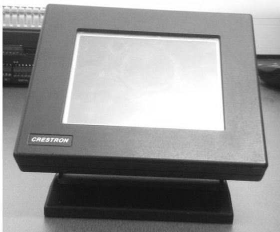
Figure 4 Touchscreen unit pulled from the Crestron control system
