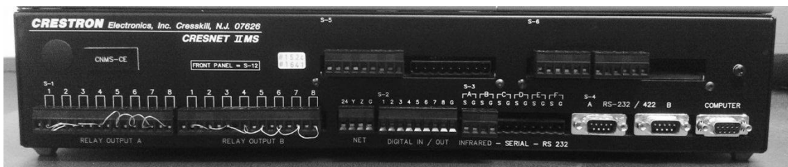
Figure 3 Back of the Crestron control unit
