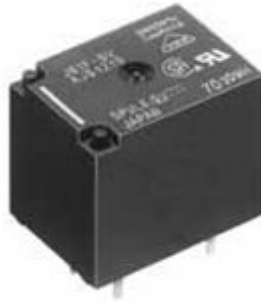
Figure 11 Panasonic JS1-24V-F relay used on the relay card.
